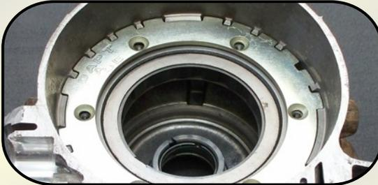
▲ Align and place retaining plate into case.
