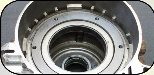
▲ Install support retaining ring into groove of case.
