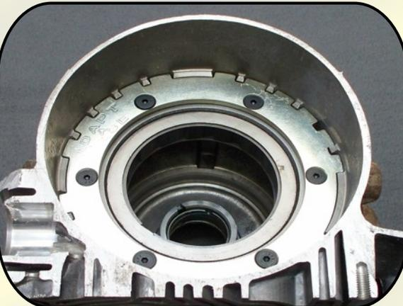
▲ Install 6 allen-head screws and torque to 100-110 inch-pounds (approx. 9ft lbs)
